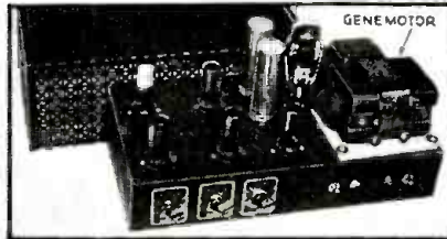
Left, a dual power P.A. amplifier, operating from either 110 V. A.C. or 6 V. D.C. Uses an 83 rectifier for A.C. and a generator motor for storage battery operation. (1203) Right, a cable type transformer for adapting low impedance mikes to high impedance circuits.
